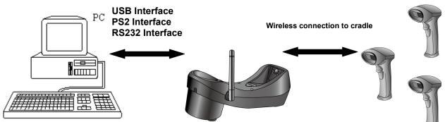
If multiple scanners are connected to the Host PC, in cradle-less mode, the data will be mixed up (simultaneous scan).
