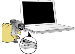
4. When being successfully connected to the dongle, the scanner will beep shortly one time with a high tone.
