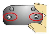
Step 5: Align the two holes on the bottom surface of the cradle respectively with the two short pillars of the iron plate for insertion of the pillars into the holes. Then, push the cradle downwards to wedge the pillars into the guidance groove.
