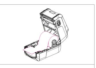
3.Pull out the print media till it pass gap sensor and cutter or peeler (cutter and peeler are optional), complete media loading
